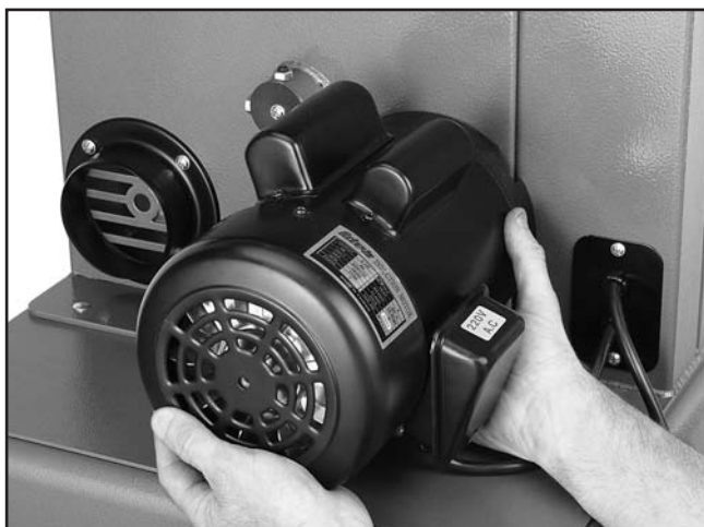
Figure 12. Installing motor (outside view).
